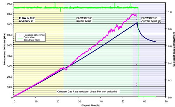
Figure 5. Diagnostic plot of GRI1 pressure response.
