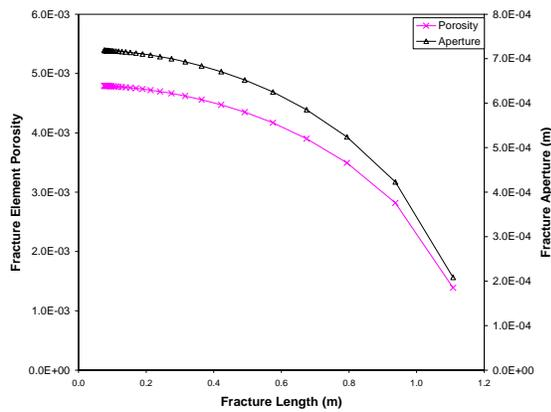
Figure 8: Estimated fracture aperture and corresponding fracture porosity using in the model.
