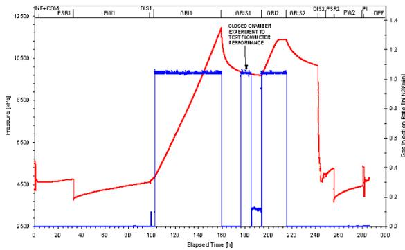
Figure 2. Pressure responses of the entire EST363 test sequence in the test zone and associated gas injection rates.
