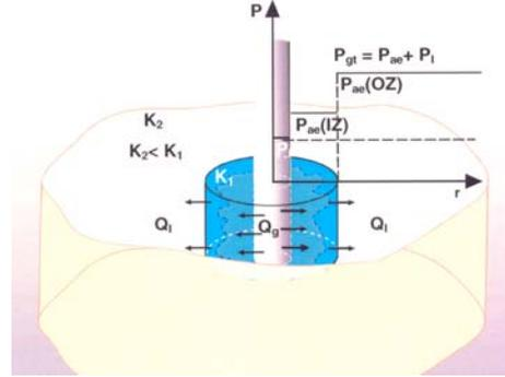
Figure 1. Schematic diagram of gas injection in a composite system.
