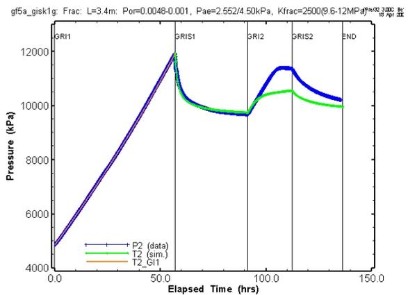
Figure 9: Simulated injection pressures for GRIS1, GRI2, and GRIS2 (calibration of GRIS1 response).
