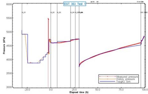
Figure 4. Simulated PW1 response incorporating borehole history.
