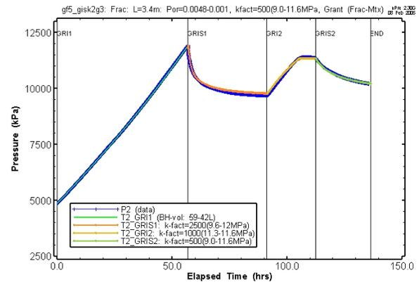
Figure 12: Simulated injection pressures based on calibration of different test sequences.
