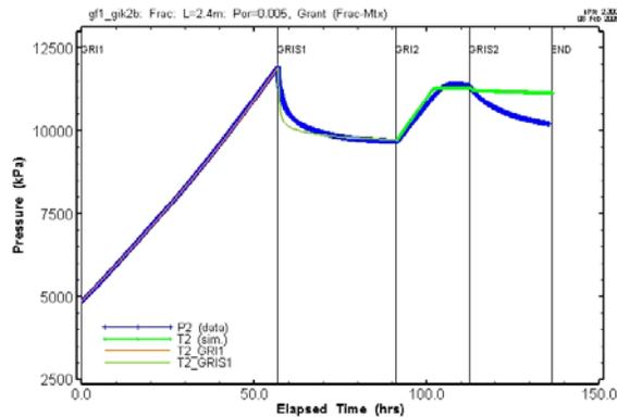
Figure 10: Simulated injection pressures for GRIS1 and GRI2 and GRIS2, assuming a “closed” fracture at the end of GRIS1..
