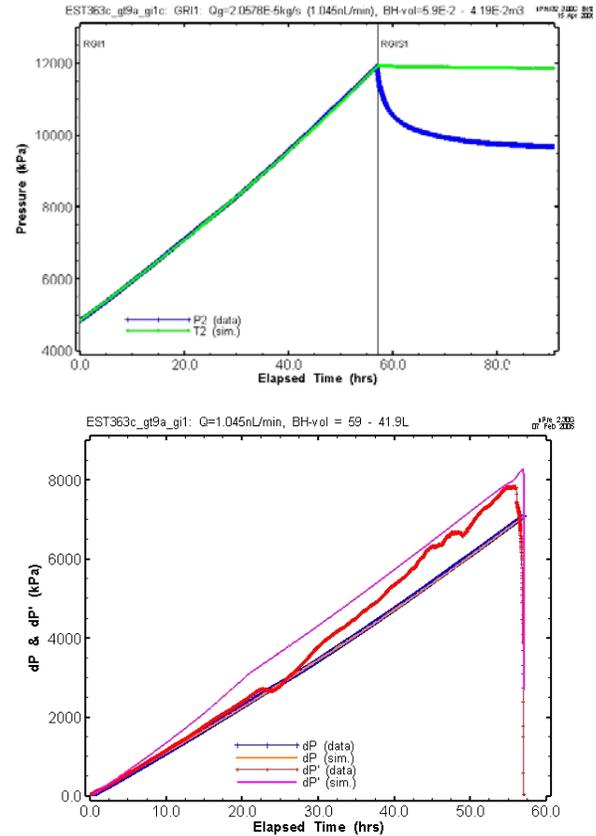
Figure 7. Cartesian plot of GRI1 and GRIS1 (top) and diagnostic plot (bottom) of the simulated and observed GRI1 response.
