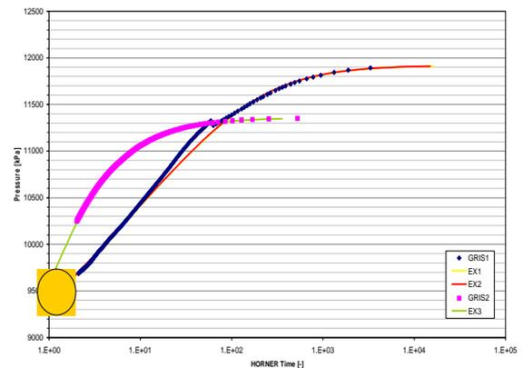
Figure 6. Horner extrapolation of GRIS1 and GRIS2 pressure recoveries.
