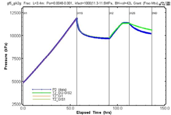
Figure 11: Simulated injection pressures for GRI2 and GRIS2 (calibration of GRI2 response).
