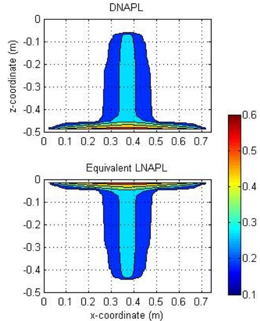
Figure 1. Simulation of downward DNAPL (TCE) migration as well as equivalent upward LNAPL migration.
