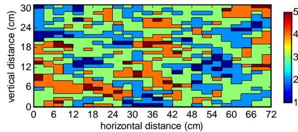
Figure 3. Lower heterogeneous zone – dark red (domain 5) is the coarsest sand, dark blue (domain 1) is the finest. In the flume, the layer is inclined 3.25°.
