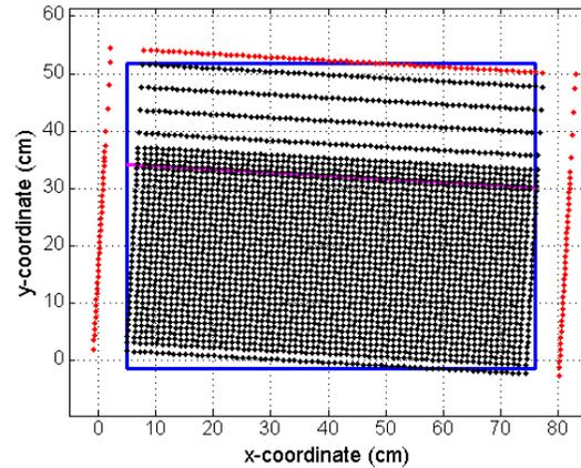
Figure 5. Centres of grid blocks used in the numerical modelling. Black: active blocks, red: const. head boundaries, blue: experiment domain, purple: sand interface.
