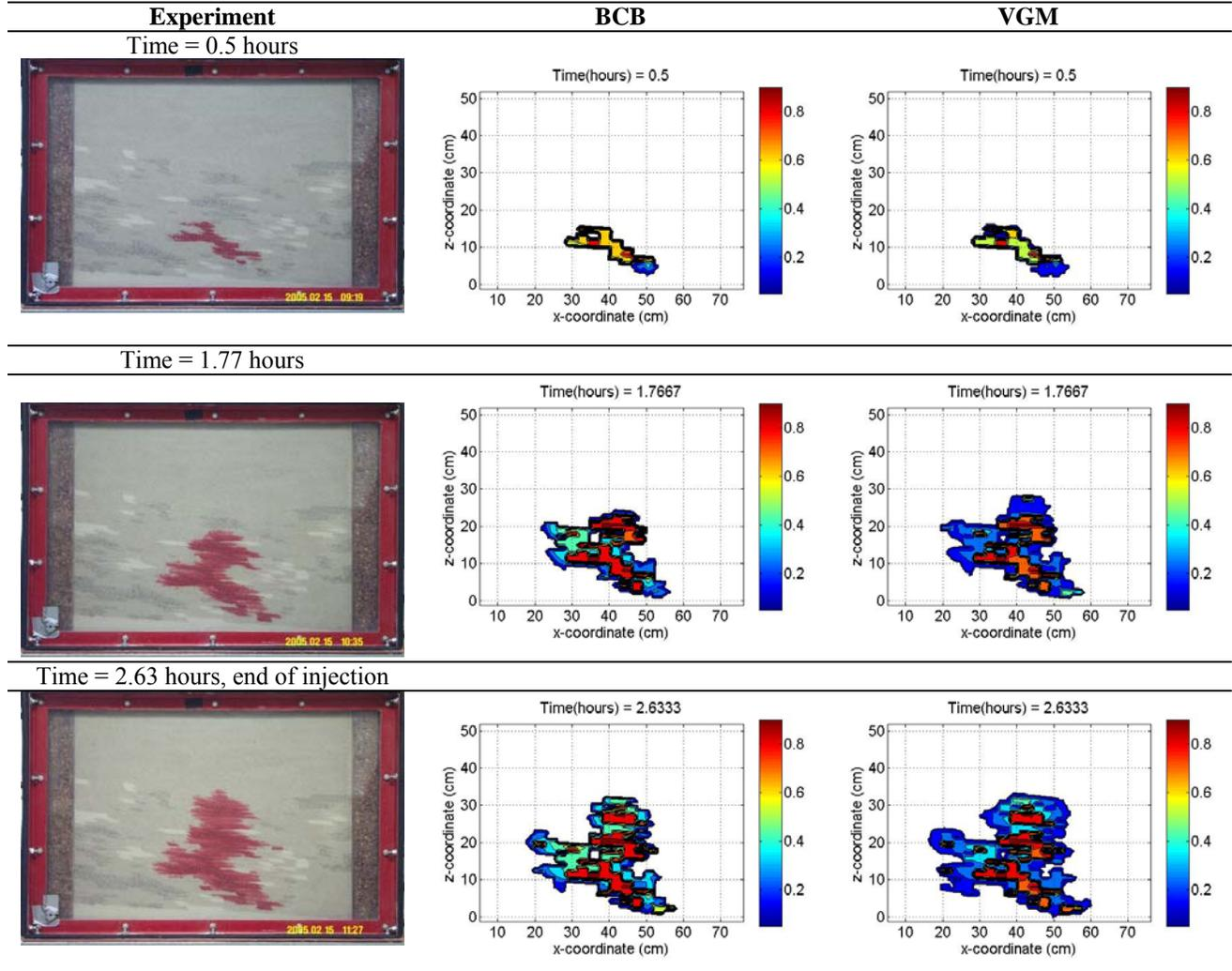
Figure 6. Spatial NAPL saturation in the experiment as digital images compared to simulated results with the BCB and VGM models.
