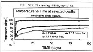
Numerical simulation showing the effectiveness of the sand filled fracture to provide a pathway for the steam is demonstrated by the rapid change in temperature at the extraction point, with steam breakthrough occurring in less than 10 days. In the clay, at 1.3 ft (0.45 m) above and below the fracture significantly longer times are required for heating to occur.
