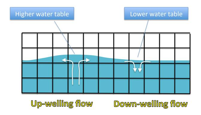
The pressure of both two-phase cells is the gas pressure, independent of the "level" of water in the cell.
