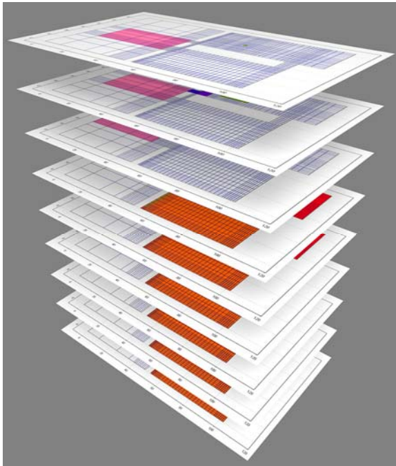
Figure 5. 2-D multiblock geometry representing the structural model in layers; discretization with a "Scottish" mesh pattern for local mesh refinement, an intermediate step before obtaining the 3-D multilayer mesh.
