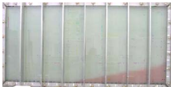
Figure 2: Saltwater positions at 90 minutes after the start of experiment with \Delta h = 10\text{mm} from the (a) first and (b) second experiment
